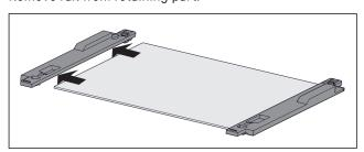
Fig. 151 Glass shelf with retaining part
