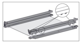
Fig. 150 Glass shelf with rails and retaining parts
